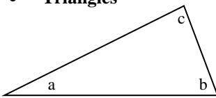
Sum of the angles in a Triangle = 180^\circ a + b + c = 180^\circ
